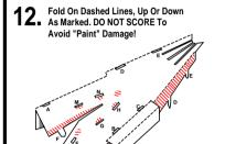
Push All Bottom Tabs Through The Matching Slots. Apply A Light Coat Of Glue To The Hatched Area. Pull Tabs Tight, Hold
